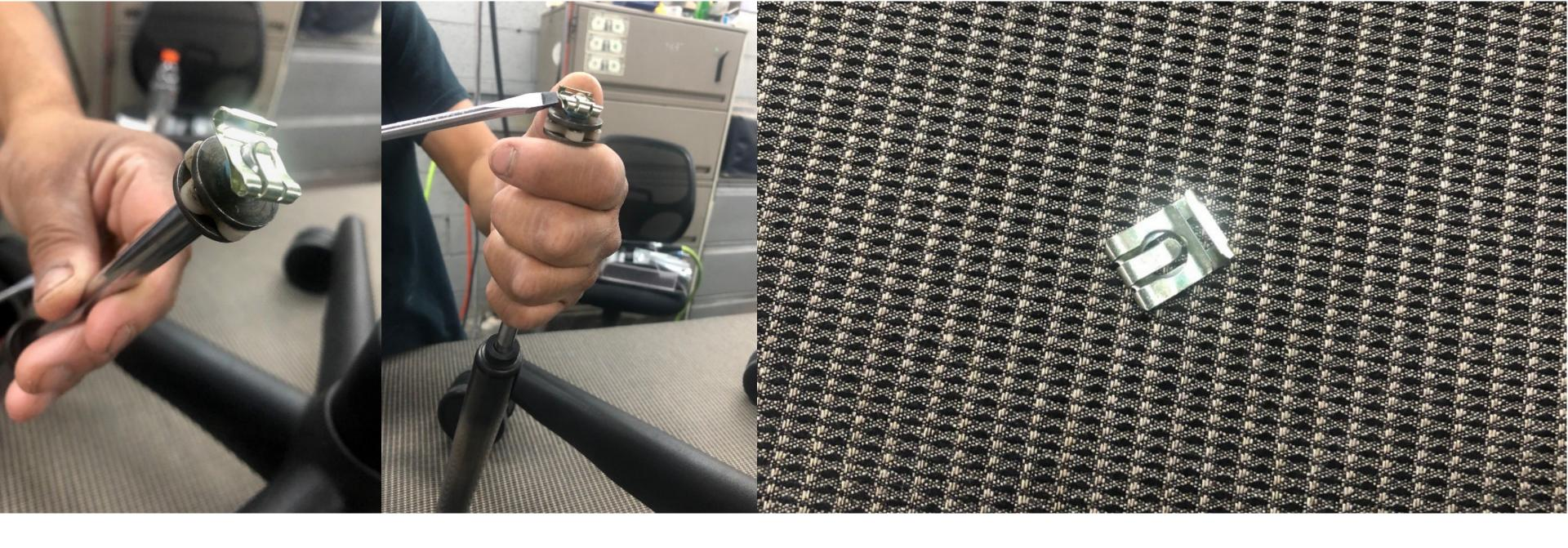
Grab the pneumatic cylinder and screwdriver.
