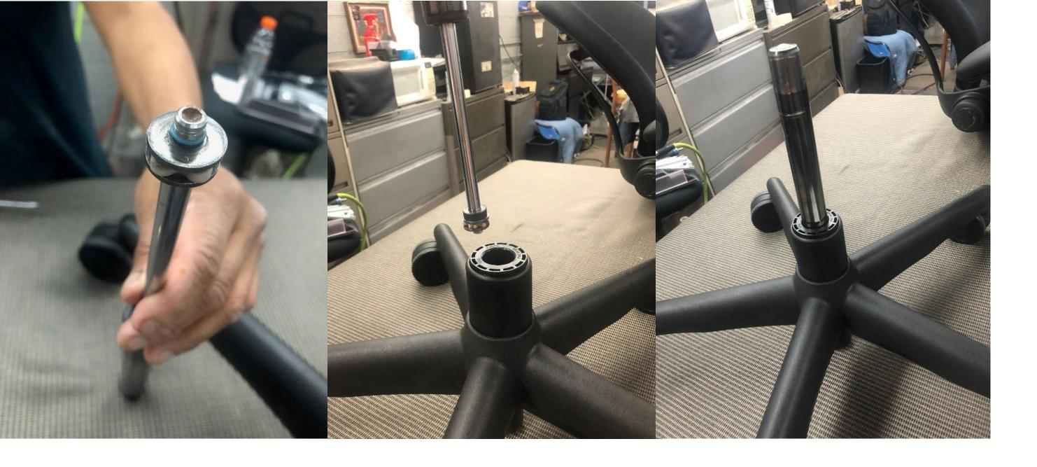
Insert the screw end of the cylinder into the 5-star base carefully.
