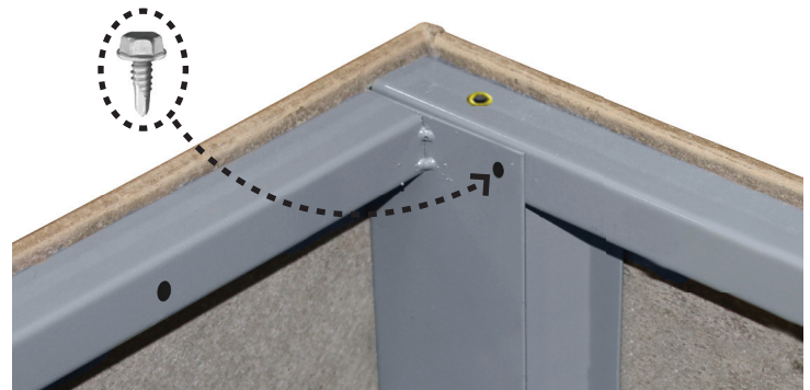
Fig. 15 Installing Self-Tapping Screws Into Panel
