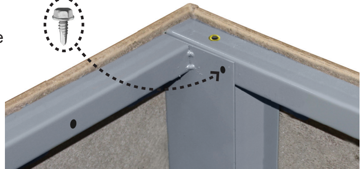
Fig. 25 Installing Self-Tapping Screws Into Panel
