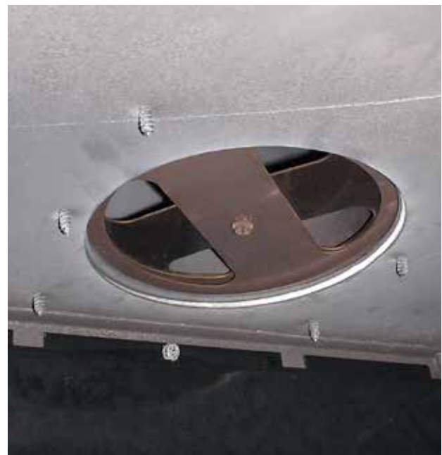
Figure 9 - Restrictor disc (shown with 2 discs closed)
