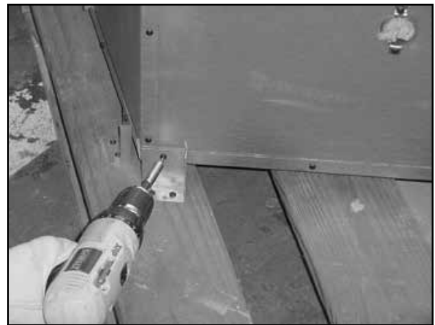
Figure 3.12 Removing Shipping Brackets
