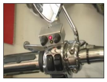
always on. The bottom LED, which is yellow, during normal operation, is on when the legs are up, and it is safe to lower the legs, and it blinks when the legs have been authorized to deploy on the next stop (more about this later!).
