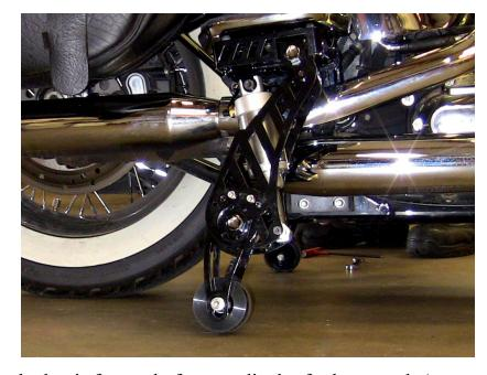
The stability of the GEN II LegUp system, relies on the pneumatic
