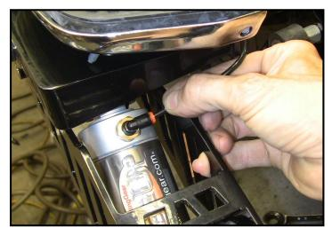
We need to route the air lines from the cylinders to the area near the left saddlebag. You should find 2 long air lines of identical lengths. On the right side of the bike, press one end into the fitting on the back of the air cylinder. These press in relatively easy, but a small tug will make sure the line is seated.
