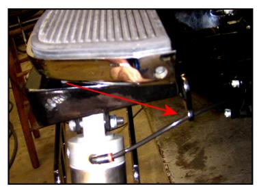
On the Left side, install the line through the hole in the mount, then into the cylinder as shown at left.
