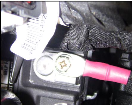
Assuming you got the cover loose, slide out the left side just a bit, so we can finally see the positive battery terminal. Carefully remove this screw from the battery. Find the 2 hoop connectors on the wire harness.
