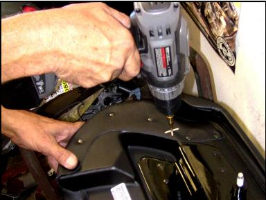
The next step is mounting the Control Switch Box.
