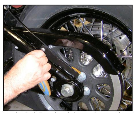
hold the bracket steady and slowly rotate the wheel. Every time a bolt passes the sensor, the light should get bright, and turn off after it passes.
