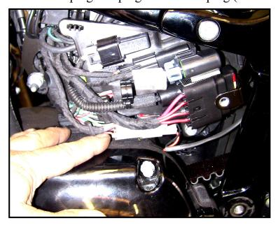
If everything went according to plan, you should have all plug connectors under the seat plugged to their matching plugs, the positive battery lead (with fuse holder) should be connected to the positive battery terminal, there should be a wire attached to the frame for ground, and on the left side you should have two big plugs waiting for a home (hanging off the fender strut), and the proximity bracket and sensor, with no place to go quite yet!
