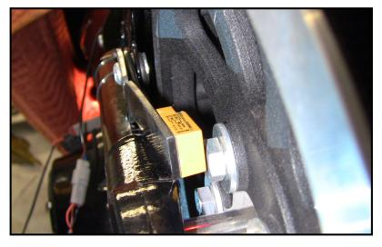
If this is not happening, you may need to get the sensor a bit closer to the bolts (5MM is a very small distance!). If you have to move the sensor closer, you may have to bend the bracket a bit. No matter what you need to do, you MUST make sure that as the wheel turns, the light works as described above! Once you are certain, tighten the bolts and test again! The automatic retraction of the legs as well as their deployment RELIES on this sensor being placed perfectly!
