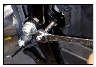
Once this is installed, we want to put a lock washer and a nut on the back of the stud, sticking out behind the frame casting. To make sure the nut is as tight as it can be, hold the nut on the outside of the casting
