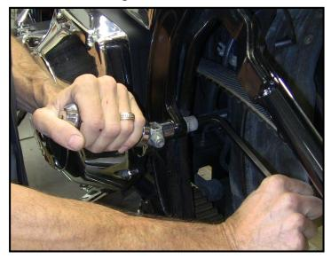
pegs. Using an Allen wrench as shown below, hold the peg on a slight angle for leverage, and loosen, the Allen bolt, and remove the pegs and the bolt.
