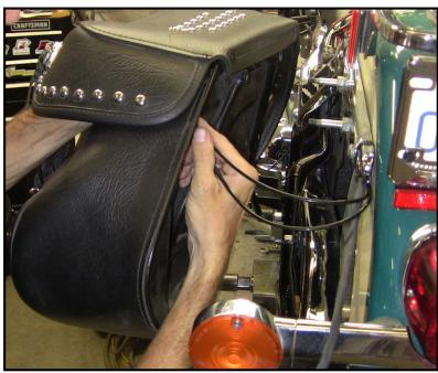
Install and tighten the mounting bolts inside the bag, and install an acorn nut on the stud from the rubber isolator. Make sure the bag mounts are tight!
