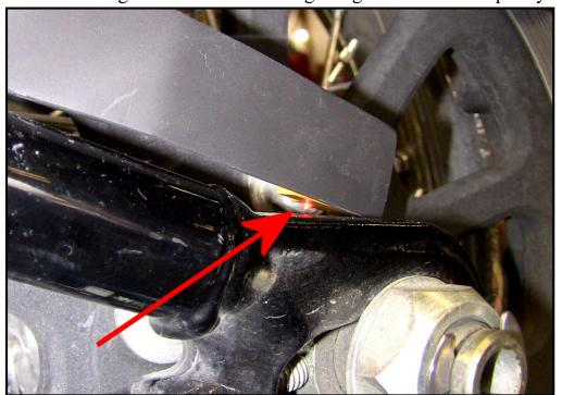
with this by rotating the wheel back and forth while holding the bracket in place. Once you feel you have the right place, hold the bracket steady and slowly rotate the wheel. Every time a bolt passes the sensor, the light should get bright, and turn off after it passes.
