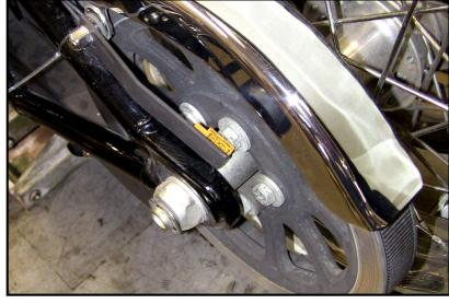
the sensor aligns near the pulley bolts. Adjust the bracket so the main part of the sensor is aiming at a pulley bolt and is centered on it (you may have to turn the wheel to do this). What we are looking for is for the LED to go bright and OFF as a pulley bolt passes the sensor. Play
