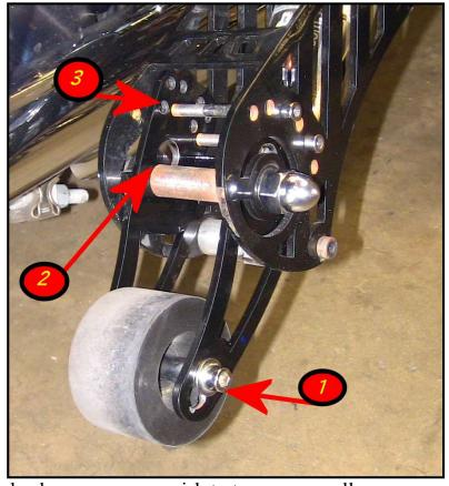
Whatever you do, try to keep the wheel holder under the leg when the legs are extended as much as possible. Rotating the wheel holder too far back lends leverage, and makes the system much less stable.
