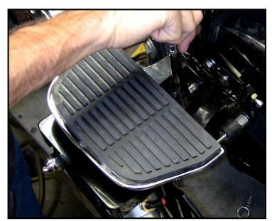
Give it a tug; it should be very stout! The left side should look like the picture (below right). If so you can install the other side the same way. The right side is a bit tighter because of the exhaust. We suggest a clean rag over the exhaust below where the leg mounts to avoid scratches.
