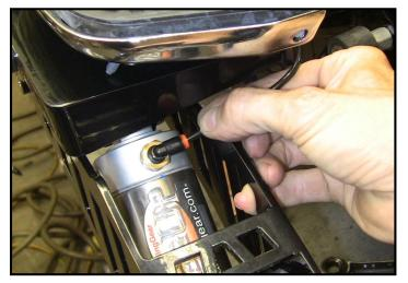
hold the line where we need it before it goes into the battery area. Don't over tighten the wire ties. Once in place, manually push the leg down and allow it to retract a few times making sure the line stays away from the pipes.
