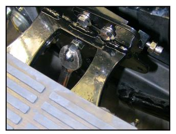
Give it a tug; it should be very stout! The left side should look like the picture (below left). If so you can install the other side the same way. The right side is a bit tighter because of the exhaust. We suggest a clean rag over the exhaust below where the leg mounts to avoid scratches, and using a ratchet to tighten the mount bolts instead of a wrench (right, below).
