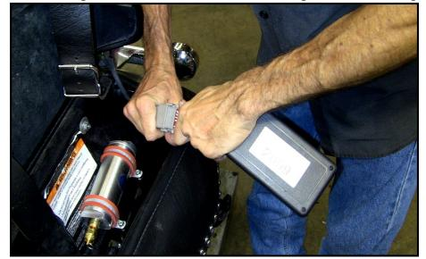
with its placement, find the computer and plug it into the 12-pin plug you kept above the top of the compressor while installing.
