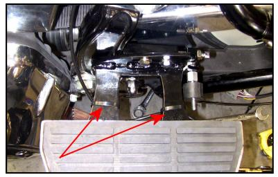
Again run the leg up and down multiple times to make sure the line does not bind. No exhaust on this side, but the belt could eat through the hose in an instant. Once you are sure the hose is clear, we need to run it up behind the oil tank and join it with the other hose and ultimately tie it to the wire harness we installed on the fender strut.
