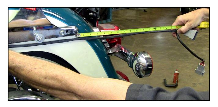
Find the proximity sensor and its three pin plug. Run the wire (plug first) through the same spot you ran the 2 plugs through, but from the fender into the area under the seat, so you can plug the 3-pin plug into its mate under the seat. Leave the sensor and its mount dangling for now; it will be mounted later.
