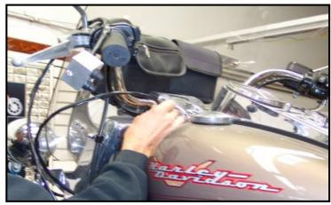
into the opening. The wiring details are found on the next page. Be VERY careful to get the wires in the correct hole; all the colors match to the mating plug!
