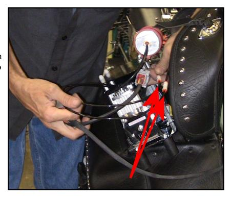
Tilting the front of the compressor system up, carefully lower it into the saddlebag, allowing it to settle into a spot as far back as it can go. The compressor should feel secure where it sits; the rubber straps around the air tank should keep it from wanting to tip. Assuming you are happy
