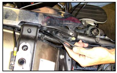
bike. Next, measure 10 inches back from the 12 pin (biggest) plug and mark the wire. We are trying to make sure we have all the wire we need but not too much extra. We chose to tie this wire loosely under the fender brace for now. We will be adding the airlines and getting all of these in the saddlebag later, as well as pulling the extra slack back under the seat.
