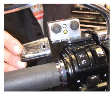
Run the wires down the back of the handlebar along with the other wires, in front of the triple tree, then under the tank.
