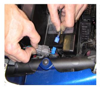
Find the orange wire with the blue plug and the black wire with the hoop connector (On later harnesses, the Black wire is eliminated). The system draws very little amperage; we decided to use the running light circuit, which is a red wire with gray traces on the grey plug you see here. We don't care where you get your 12 Volt source as long as it is switched and stays on while the bike is running.
