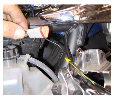
Here we show the plug under the seat and have a temporary wire tie on the frame so the wire can run down to the left back axle area for mounting later!
