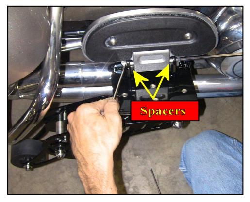
on. This replaces the rubber we removed from the floorboard mount!
