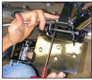
we don't need the rubber when we are done, so don't worry if they get damaged during removal. We want to expose the two holes the rubber is filling, to be used to mount the Leg Assemblies.
