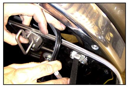
We actually should have cut this notch a bit more forward toward the metal bracket you see here. Position is not critical, but the lines and wire go into a notch on the compressor top later, and a bit further forward makes this a bit easier.
