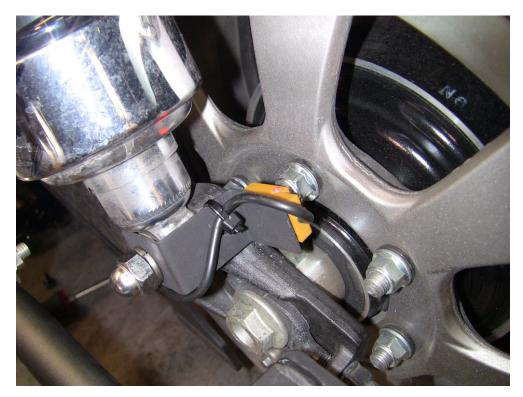
Slide the bracket on the shock bolt and reinstall the lock washer and cap nut with a bit of Loctite. Do Not tighten completely yet. The bracket must be rotated to the proper position for it to work properly. Notice the orientation in the picture here; we want the bolt to cross over the middle of the leftmost area of the face of the sensor.
