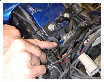
Now run the wire with the 2 big plugs on it, down the left fender support toward the back of the
