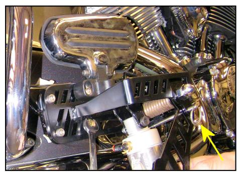
Tighten all 3 bolts a bit at a time using a long Allen for the rear bolts and an open end wrench for the bottom front bolt (left). It is easier, once the lower bolt is started, to tighten the rear bolts and the rear floorboard bolt, then remove the pin holding the leg down, and tighten the bottom bolt.
