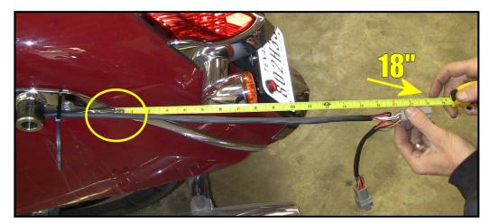
Find the two BIG plugs on the harness (12-pin with an 8-pin pigtail attached), and measure 18" from the point of the fender support to the 12-pin plug. We need this amount of wire to be able to go into the saddlebag.
