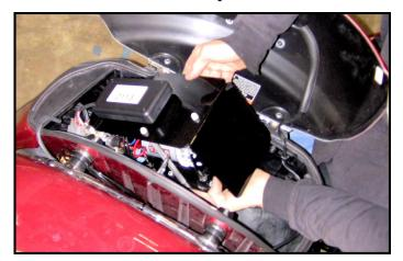
Tilt the compressor system back as shown here, making sure the two plugs are moved toward
