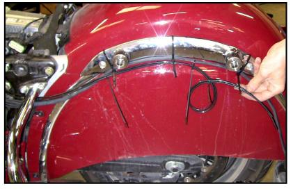
Notice the loop in the air lines shown here. We need about this amount of line in order to have the ability to remove and re-install the bags.
