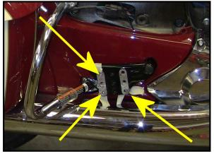
At left is a picture of the floorboard mounts with the boards removed (right side). The arrow shows the holes we will mount the legs with. To simplify the installation, find (4) 5-16" Lock-nuts, insert them into the castings behind these holes, and use masking tape to hold the nuts in place during the mounting process.
