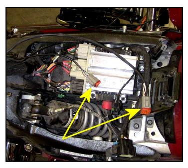
Due to global distributions problems, we may have to use a four pin plug instead of a 3 pin plug. The colors still need to be the same across the plugs with pin 4 empty!
