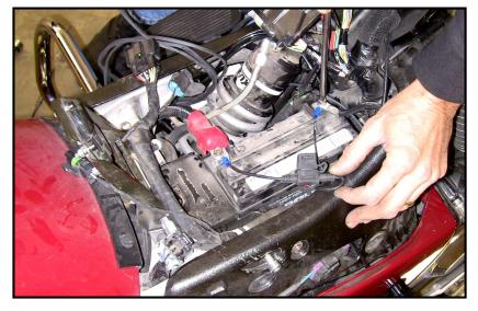
This wire should be run around the front of the shock to avoid the springs. The single wire with the fuse holder gets attached to the positive terminal of the battery, the other to the negative. Remove the fuse for safety before connecting the positive wire.
