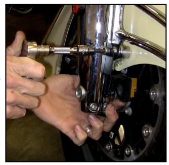
bolt is too short, one of the floorboard mounting bolts you removed earlier can be used as it is ¼" longer) Tighten this bolt with the bracket placed as shown in the picture below.
