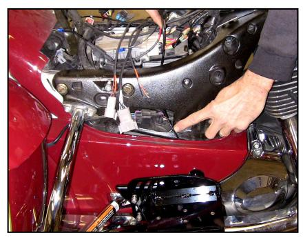
cover if you find it easier. A wire-tie to the bottom of the mount to keep the line away from the pipe is a good idea here!
