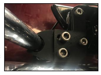
The mount works by offering resistance against the floorboard bracket twisting on its mount bolt. The bottom of the rear mount will NOT allow the back of the whole assembly moving up, and ultimately keep the entire part less likely to loosen over time.
