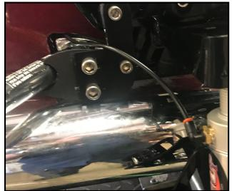
Notice that the airline (covered later in this manual) lies on top of this mount, rather than through the center bolt hole (hidden by this new mount). We ultimately tie it gently, putting a wire tie through the top slot of the brace just installed.
