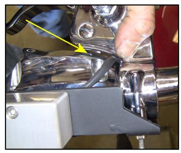
already removed, and how we tied the wire off to the brake line on its way up to meet the other wire. Leave the Proximity Bracket dangling for now as seen here.
