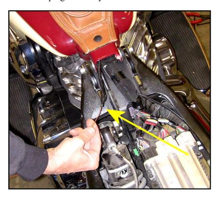
The picture here shows the two plugs reassembled in the under seat area. We will connect these in a bit and show you how we need to stow these wires for safety later. Note the detail pin-outs in the lower diagrams. Now on to the wiring harness!
