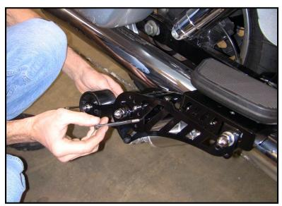
On each supporting leg, you should find two bolts down near the end, by the wheels. The two bolts control the angle of the 'Wheel Holders'. By moving the wheel forward or back, we can tailor the length of the support arms to a particular bike.
