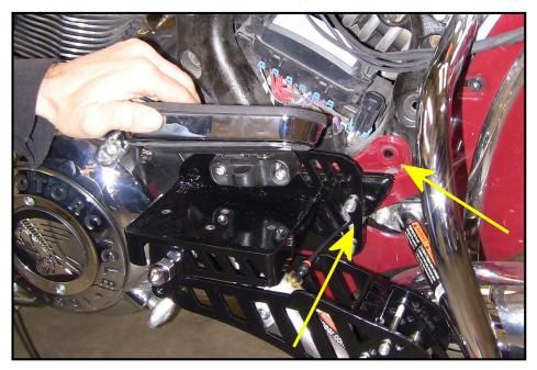
On the left side, we need to remove the two top bolts in the side cover and loosen the lower bolt. We need this loose to make sure the line can get where it needs to without binding. Once this is done, attach the line to the cylinder, run it under the mount and under the side cover where the crash bar mount attaches to the bike.
