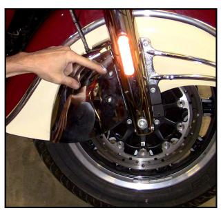
Turn the ignition switch to the on position. The LED may or may not be on. What we are looking for here is for the LED to light as a rotor bolt passes close to the sensor and to go out as the bolt passes by. Have someone watch the LED as you roll the wheel, or the bike, back and forth making the bolts pass close to the sensor.
