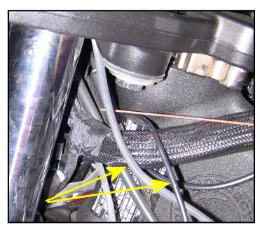
Next, we tied the wires from to the end of the rod with electrical tape, and gently pulled them under the seat. The picture below shows where the wires emerged. Once complete, we removed the tape and re-assembled both plugs carefully.
