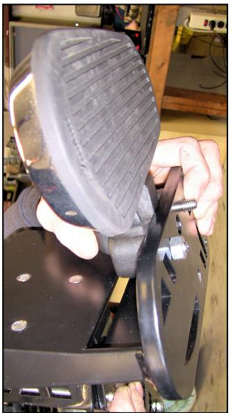
Apply red Loctite to the threads of the bolt and reinstall it. Make sure the bolt is **VERY** tight. These boards will have a tendency to pivot on this bolt if it is not tightened properly. We suggest that ANNUALLY, you remove the Leg system and retighten and lock these bolts as a preventative measure.
