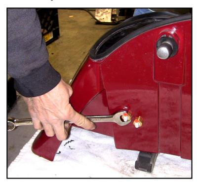
Once the bottom fitting is in place, install and tighten the top fitting. Now the bag is ready!
