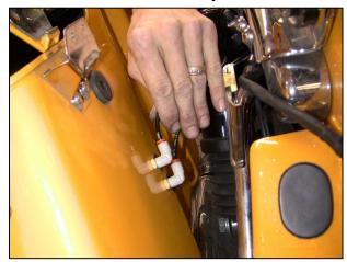
The last thing we need to do is create a small notch for the wires to get through when the bag is closed. We use a rotary burr, but you could use a file or a small saw, to cut the notch you see here.
