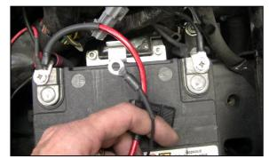
This wire should already be under the seat area. We want to connect the wire with the fuse holder to the positive terminal of the battery (the battery cable should attach closest to the battery with this connector and any others attached after the battery cable, as shown here). Plan where you want the fuse holder so you can get to it if it is ever required!
