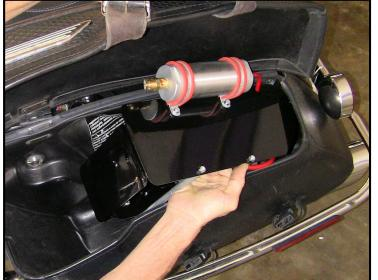
The picture at left shows us starting the compressor into the bag. As we do this, we take the two air lines with male-male fittings attached and start it through the hole you drilled into the bag.
