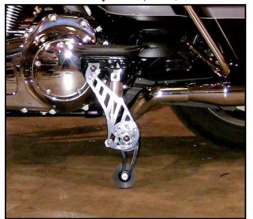
should look like something like this. Also notice that the floorboard is level. We have seen one bike that had floorboards that leaned forward, which would **RUIN** the geometry required here. Please verify that your floorboards are level!
