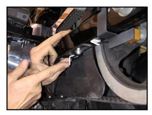
Tie the Proximity sensor wire down the left side of the swing arm for pulley bolt bikes, or the right for Cush drive bikes. Use the supplied self-adhesive tabs, to secure the wire snugly to the swing arm. Just make sure you route this safely and tie it off securely! Finally pull all the extra wire under the seat area.
