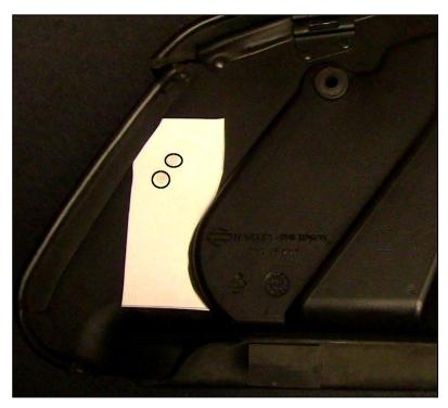
First we need to find, near the end of the manual, the drilling template for soft bags. Carefully cut this template out, and tape it to the inside of the left saddlebag, as seen in the next picture. The flat bottom of the template lines up with the bottom of the bag, just before it turns under, while the curve should fit nicely as seen here. The upper left angle should fit inside the line where the leather meets the hard back.
