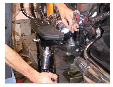
Take the other line; insert it into the left cylinder as you did on the other side. Mark the far end as 'LEFT' and tie the marked ends together with masking tape, so we can run them together.
