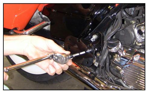
Each leg has two pieces; we have a mount that attaches directly to the bike and a leg that mounts to this piece. This new mounting system is **MUCH** stronger that Harley's floorboard mounts.
