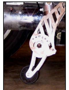
The first picture (above) shows the setup for standard height Harleys. The boards are set in the highest position, the wheel holder is set with the strap facing up and the small bolts set in the second and fourth hole from the back of the leg (Notice curve of wheel holder). This is how we should have sent the legs to you if you told us you bike was at stock height!
