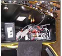
Once the compressor is in place, the air lines should be attached to the fittings you mounted in the saddlebag.
