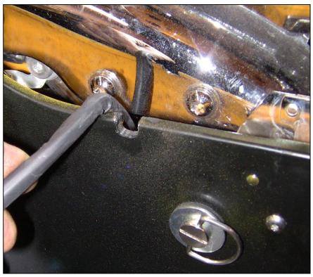
holds the bag on) is where you want to place the relief. A bit left or right makes little difference, but this wire goes down into a relief cut in the top of the compressor cover, so the more accurate you are here, the better!
