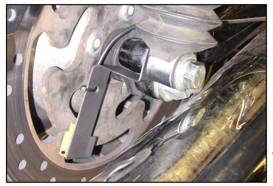
If this is not happening, you may need to get the sensor a bit closer to the brake rotor (5MM is a very small distance!). If this is not happening, you may need to get the sensor a bit closer to the brake rotor (5MM is a very small distance!). If you have to move the sensor closer, you may have to bend the bracket just a tad (you may even need to loosen or remove it to bend it as you need to). No matter what you
