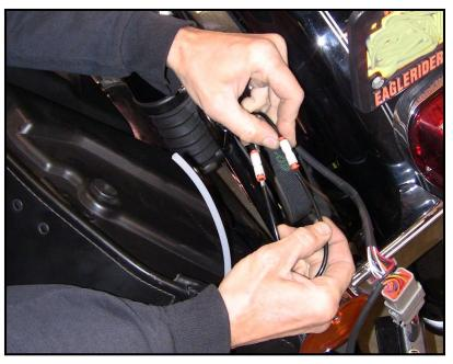
We need to find the inline connectors (white in this picture, could be a different color) and attach them to the end of the lines you ran toward the back of the saddlebag.
