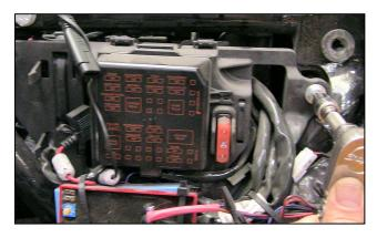
The next step is to route the wiring harness. The harness and the plugs are routed mostly under the seat. Different models have different amounts of space in this area, and all the wires are long enough to allow you to place the connectors in the best place for your bike.
