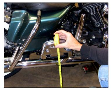
Measure this from the small donut on the bottom of the board mount in the center of the board with the bike held level (we set the bike on a jack here, but you can have someone try to hold it upright if need be). We suggest taking this measurement from both sides and dividing them in half. Armed with this info, we can use the list below to find a good starting point to set the wheels up properly!
