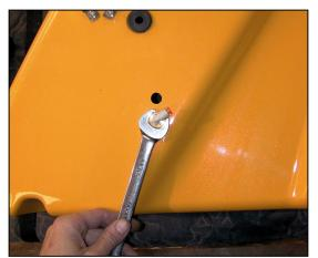
Start with the lower hole, and tighten the fitting. No reason to make it too tight; there is no chance for leaks here, and the elbow spins to make it easier to attach the lines.
