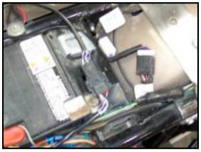
general area and plan where you would like to tie them up safely. The Proximity sensor is not mounted yet because we need to have power to make sure it is placed perfectly, so just route the wire for now. You can collect any excess wire under the seat area, when the time comes.
