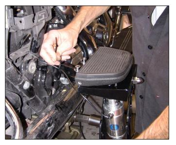
just be sure that it is secure, and cannot be damaged by anything hot or moving. Once run, you should mark the end with masking tape as 'RIGHT'.
