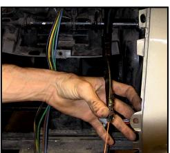
tape those hoses and the wire ends to a lead wire (we use welding wire), and run it through as
