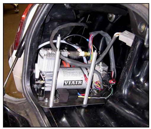
Here is a picture with the compressor in its' final resting spot (without the top). We want to pull the extra line and wire into the area above the compressor. When you are done, we would like to make sure that the hoses are not resting on the fins of the compressor (they can get warm!). We will put the top on later to make this all pretty.
