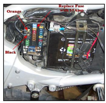
present) gets attached to the lower post. Notice that the wires can be routed out of the fuse box to the left where there is a relief for each. We strongly recommend that you replace the existing 5Amp fuse (second one down on the left) with a 10 or 15AMP fuse. This fuse only supports the orange wire here and a 5 amp fuse is just a bit too light. These connections are only on when
