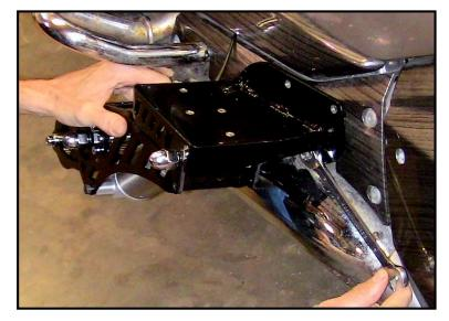
Make sure you use Loctite on the bolts and check them frequently for tightness. It may be easier to have an extra hand supporting the assembly, as it is a bit tricky getting to the two bolts. Repeat the procedure on the other side of the bike.
