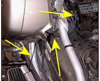
which (We may have marked one of them with tape!). Take the marked line and run it to the right-side cylinder as shown. This route keeps the line away from the pipe and anything else that may damage it. Once it is run, attach the end to the cylinder. It is easier to pull the leg down to install the line as shown below. These lines just press into the fittings. Once inserted, give the line a tug to make sure it is staying put! Next, run the
