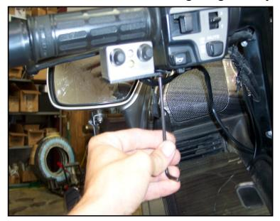
Using the bolt provided, slip the bolt through the black plate and spacer, and then thread it into the switch housing. This bolt needs to be snug as when the buttons are pressed, we don't want the housing to pivot on the bolt (picture left). Square the box before tightening the bolt. Route the wire down the handlebar and leave it loose near the front forks to be routed under the seat with the proximity sensor wires. Use wire ties to hold the wire to the bar.
