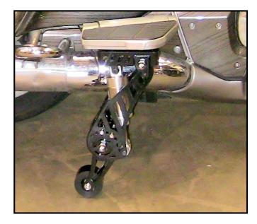
PLEASE NOTE: The GEN II system is bike height sensitive, and Gold Wings can sink when loaded two up. You should test the stability of the system with a passenger and adjust the air shocks to stiffen the suspension and get the stability you have here with a rider. You may need to re-adjust the shocks for solo riding as well.
