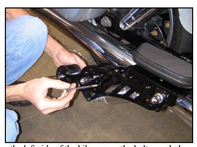
On each supporting leg, you will find two bolts down near the end by the wheels. The two bolts control the angle of the 'Wheel Holders'. By moving the wheel forward or back, we can tailor the length of the support arms to a particular bike.
