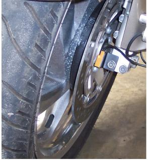
The LED on the sensor should be off when no bolt is passing the sensor, and the LED should light when a bolt passes by the sensor. Play with this by rotating the wheel back and forth while adjusting the bracket in, out, left or right until the light blinks consistently.
