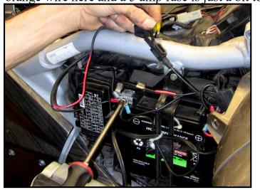
The other wires attach directly to the battery. The one with the fuse holder is attached to the positive post (we suggest removing the fuse for now!), and the black wire to the negative. These power the compressor through a relay! Notice the route of the wires underneath the frame rail.
