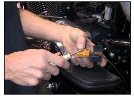
The next step requires some care. If the bike is still on the lift, have a helper hang on to it as you touch the left button for just a split second. The legs should move down, likely until the wheels hit or miss the lift, and they do this **VERY** quickly! The compressor will likely start and run for about 10 seconds. Press the left button again and they should move up.
