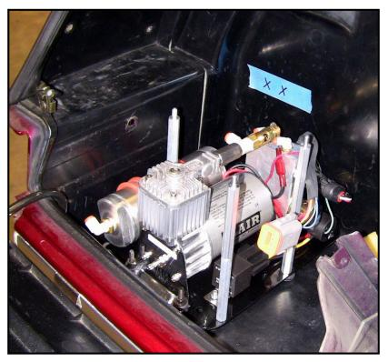
As shown here by the tape with the two 'Xs' on it, we want the holes an inch or so above the round rubber circle in the inside of the bag, about 4" or so from the bag bottom. You can drop the compressor in to compare the locations. Exact placement is not critical; just try to get the holes about where you see them here.
