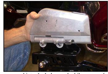
spacers, and into the holes on the bike exposed after removing the floorboards. We suggest the front bolt be installed first, and then you can lower the leg against its spring to install and tighten the rear bolt.
