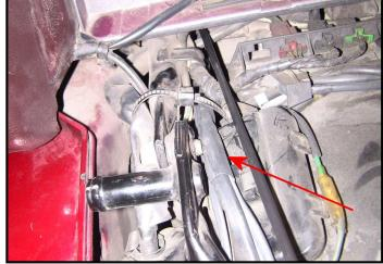
Once the tape is removed, we can reassemble the twelve pin plug (See 'Illustrations' toward the end of this manual for diagram. IT IS CRITCAL that you assemble the 12-pin plugs, from the saddlebag and from under the seat, EXACTLY as it is pictured at the end of the manual), and just leave the air lines dangling for now. The picture above (left) shows the wires and lines. The ones 'From Saddlebag' will be covered later.
