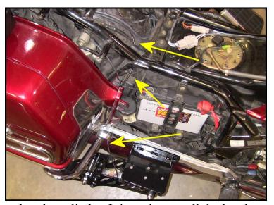
We need to route the air lines to the cylinders; this way we can protect the excess, and ultimately pull them into the right saddlebag.
