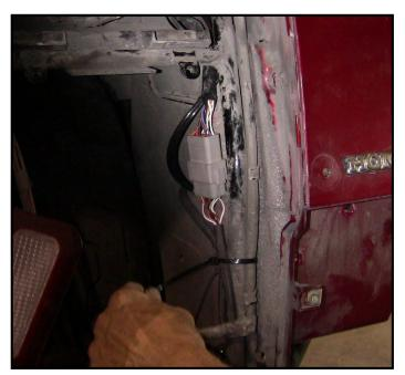
The area under the trunk was next. We connected the plug and tied it off high so it was away from the spinning tire and any water it might kick up. The plug is water tight, but no reason not to be thorough.
