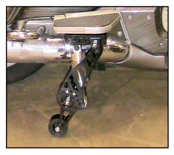
PLEASE NOTE: The GEN II system is bike height sensitive, and Gold Wings can sink when loaded two up. You should test the stability of the system with a passenger and adjust the air shocks to stiffen the suspension and get the stability you have here with a rider. You may need to re-adjust the shocks for solo riding as well.
