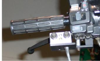
At this point we need to find the proximity sensor (yellow thing) & bracket and get the plug off the end. The wires from this sensor need to be routed from the front left fork area, up toward the handlebar, to join the wires from the switch box. Route the wires under the caliper cover if one exists, and up the fork leg.
