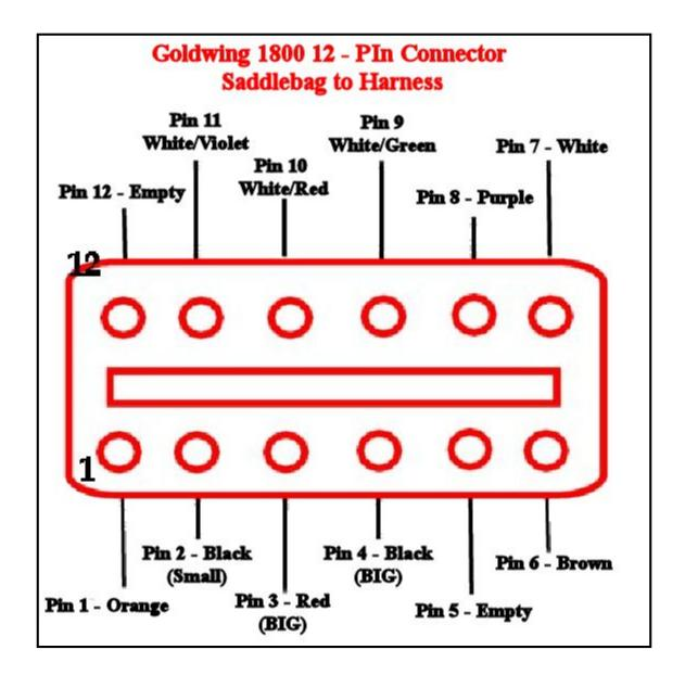
There are (2) 12 pin plugs to be assembled; the Female plug (male pins) from the harness under the seat, and the Male plug (female pins) going through the saddlebag. It is IMPERATIVE that you assemble them just this way so if you ever need support, we will know how to help! This could save you hours of aggravation.
