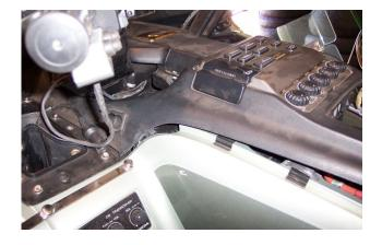
Check the pins to make sure none where damaged during the process. Make sure the wires under the fork have enough room to allow the bars to be turned and that they don't get caught on anything.
