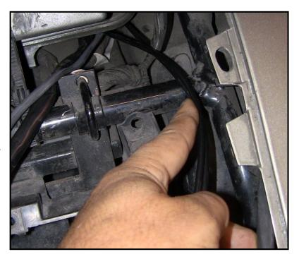
Please Note: The side covers on both sides are a bit trickier to remove with the legs attached to the bike. Removing the seat helps, but the covers will come off without this. You can also loosen the leg attachment bolts if getting the cover off proves difficult. Just remember to re-torque these when completed!
