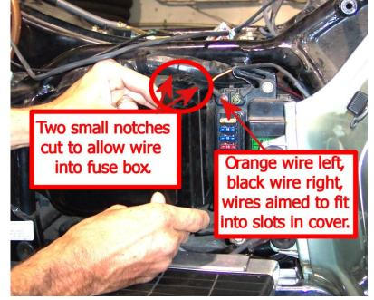
to this post. The black wire (If present) gets attached to the right post. Notice that the wires can be routed out of the fuse box by making two small notches for clearance. These connections are only on when the bike is either on or in accessory mode. (We STRONGLY suggest that you change the accessory fuse (top one) to one that is at least 5 Amps bigger than the stock one. It should have a 5 Amp or bigger; the wires can handle 20 Amp easily!)
