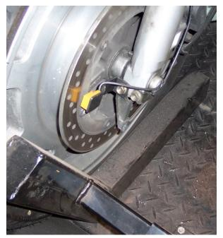
away from the bolts or closer. Look at the picture at the right. Once the bracket is mounted, turn the key to the accessory position, spin the wheel or roll the bike and watch the behavior of the sensor as the bolts pass it.
