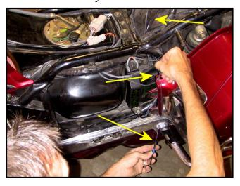
Before considering that the lines are tied off properly, put the side covers back on, and test the travel of the legs up and down, making sure nothing binds or damages the lines.
