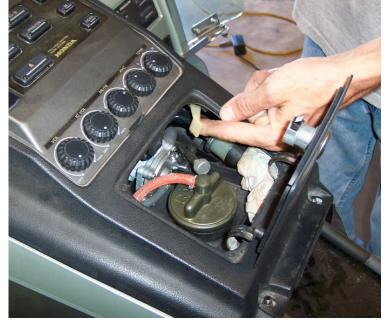
Once the wires emerge in the area under the seat, pull on the wires, making sure they move easily. If not, there is a bind. See if you can clear this bind, or pull the wires back out and start over (Sorry!). Once this works out, carefully remove the tape to expose the silver pins.
