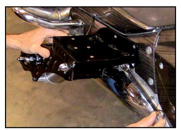
We have found that mounting the floorboards to our assembly is easier before you mount the assembly. Find the 2 5/16 X 7/8" button heads, and locknuts to match. Slide the buttons from the back, through the mount, then the floorboard and secure it with the locking nut. It should look like the pictures here when complete. You can wait until the
