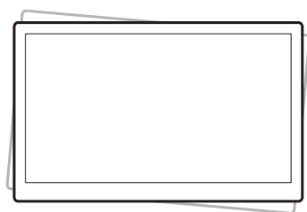
Screen Leveling (+3° to -3° Left/Right)
