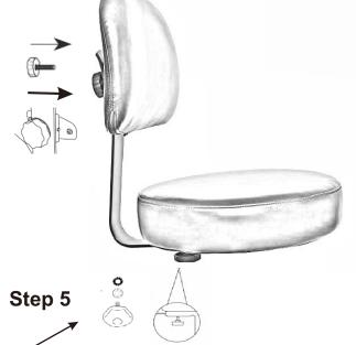
Remove (unscrew) the knob and washers from the mechanism. Insert the bottom of back bar into the opening slot of the control mechanism (as seen in the diagram above).
