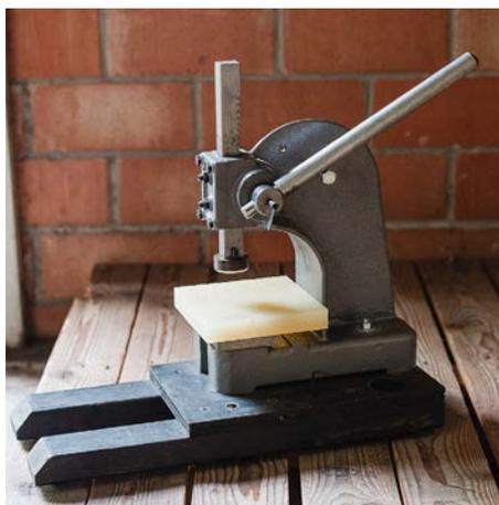
**Photo on Left:** Press is set up with die set in position.
