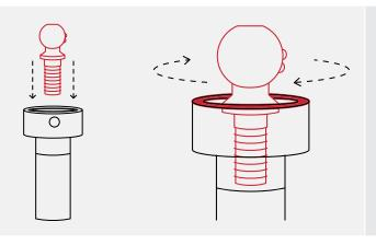
Thread the desired **Hitch Ball** into the Ball Mount.
