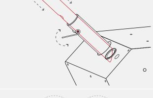
Insert the base of the handle into the **Handle Receiver Tube**.
