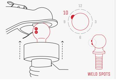
Insert the assembled Ball Mount into the Hitch and lock as normal.
