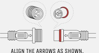
Connect the two parts of the **Handle Control Cable**.
