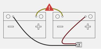
DO NOT CONNECT 80" CABLE TO BATTERY CONNECTION TERMINALS
