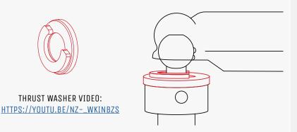
Place the **Thrust Washer** on top of the **Ball Mount Collar**, with the open section facing your trailer.
