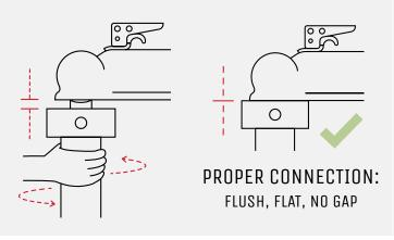
Turn the Ball Mount Counter Clockwise until the gap between the Ball Mount Collar and Trailer Tongue closes.
