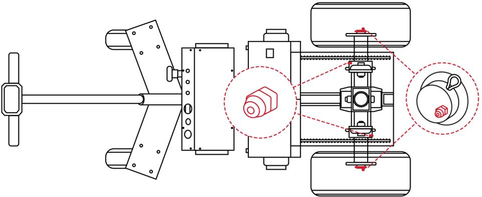
**Charging the On-Board Batteries:** Pull out on the **Battery Disconnect** to connect the batteries. Plug the **Charger Cable** into the Dolly and the opposite end into a nearby wall outlet. (Page 7)
