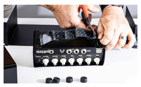
Step 3: Gently remove the Velcro adhesive protectors and place the units in the carriers adhesive side down. (The Velcro allows them to be removed and re-positioned.)
