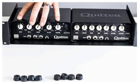
Step 4: When positioning your units inside the rack, apply pressure inwards by allowing the opposite side to "hang down" slightly then tightening the screws and pressing "up" under the bottom side of the carrier while installing the screws on the other side. This will "compress" the units in place to prevent movement.
