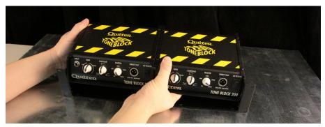
Step 5: Align the 4 screw holes on the sides of the completed 200 block series pair and loosely insert 4 screws and bolts on each side.
