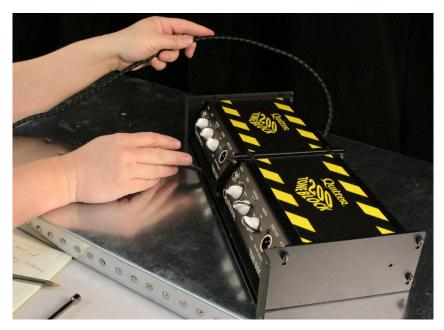
Step 2: Gently press down on the rack tray to make space for your direct out XLR cable to fit between the 200 series blocks and the Rack Tray. Go ahead and plug these in as well.
