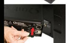
2) Insert the 1/4" speaker cable into the 4 Ohm speaker jack on the back of the amplifier.
