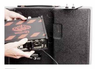
2) Insert the 1/4" speaker cable into the lower speaker jack on the back of the amplifier.
