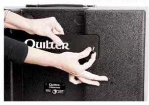
1) Remove two thumbscrews from rear retainer plate.
