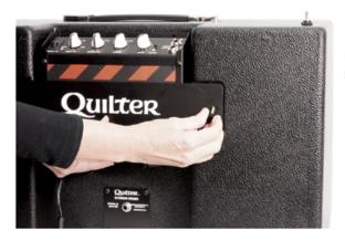
5) While holding the amplifier in with the rear retainer plate, screw in the two thumbscrews on either side of the plate.
