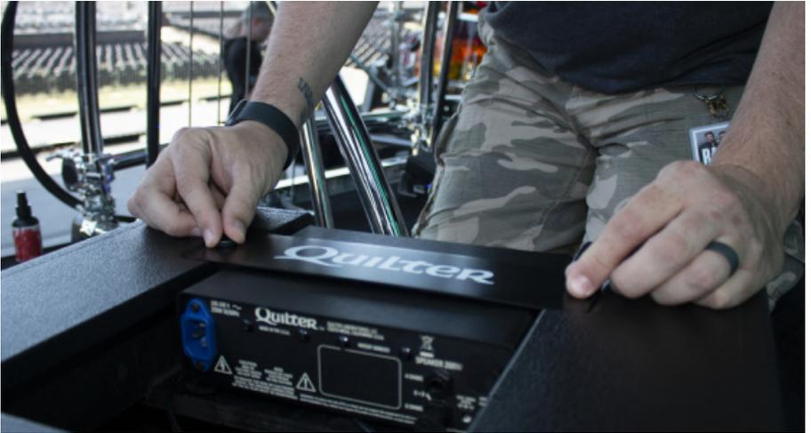
Remove the two thumbscrews on each side of the amplifier on the rear of the amplifier.
