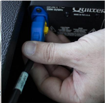
**Pro Tip:** The TT12/15 combo comes standard with a locking AC cable. When removing or re-connecting it, you may need to press firmly on the yellow button.
