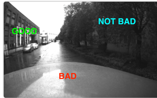
(b) Car: The hood covers almost half of the frame, preventing feature acquisition.
