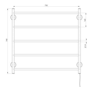
Electricity Input: 240V, 50Hz | Power Rating: 45W | IP Rating: IPX4 | Connection position: Bottom right | Connection type: Plug-in or Hardwire
