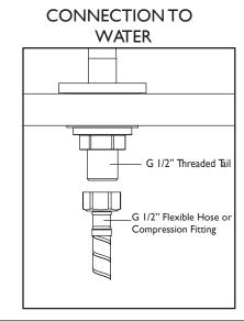
Drill a 22-25mm hole through the bench surface. Insert Outlet as shown. Fit Plastic Washer and G  $\,$  I/2" Locknut to the theaded tail. Tighten firmly.
