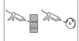
Apply small amount of silicon to mounting bracket and wall in and around the screw holes.
