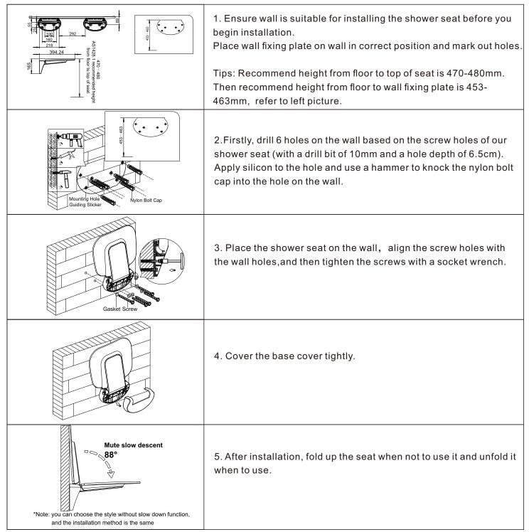
\*Note:The drilling bit is 10mm, and the drilling depth is greater than or equal to 6.5cm
