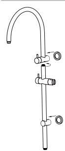
4. Locate and push shower rail assembly onto wall adaptors. Tighten grub screws firmly with allen key provided.
