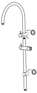
3. Screw shower rail into shower arm component. Tighten firmly. Push 2 back plates onto shower arm component and lower mounting pillar.
