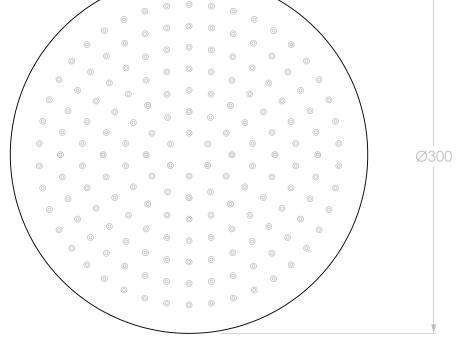
WORKING PRESSURE: 350 – 500KPA (INCLUDING COLD AND HOT WATER PRESSURE)
