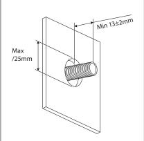
2. Apply thread tape (or similar) to the 1/2" connection, then screw the water inlet connector to the connection.
