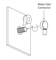
**3.** Screw the rail connector to a wall stud making sure it is vertically in line with the top rail connector. Distance between the top and bottom shower connections is 670mm.
