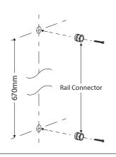
**4.** Check the grub screws are wound tight. Push the rail brackets onto the top and bottom rail connectors until they are against the wall. Secure with grub screws. Secure with grub screws.
