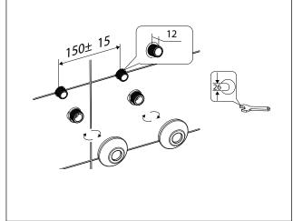
**3.** Attach the wall mounted bath set to the wall at the fixing points by pushing the wall brackets over the 2 connectors and tighten using a spanner.
