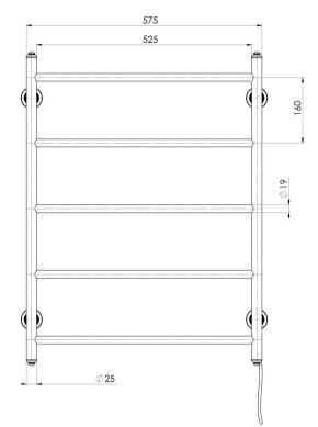
Electricity Input: 240V, 50Hz | Power Rating: 35W | IP Rating: IPX4 | Connection position: Bottom right | Connection type: Plug-in or Hardwire
