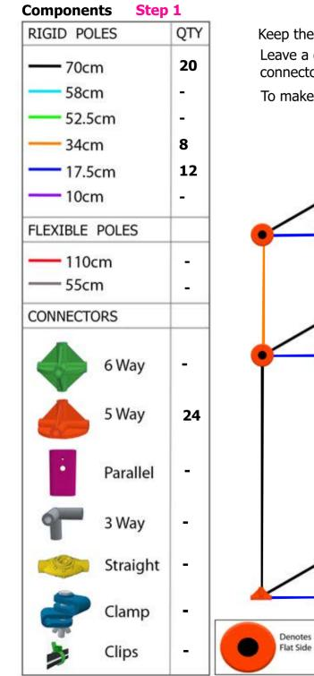
Keep the open holes of the 5 way connectors are in the horizontal plane whenever possible. Leave a distance of 105cm between the two frame bases. Use 2 x 52.5cm poles and a 5 way connector to set the correct space and remove them at a later stage.
