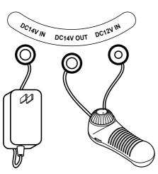
To use your machine, connect the power adapter to an AC outlet and insert the jack into the leftmost port (DC14V IN). To connect the Bullet Controller, attach the jacks of the controller into the respective ports in the machine, with the middle being the port that powers the controller (DC14V OUT) and the right port that allows the controller to change the thrusting speed of the machine (DC12V IN).
