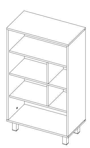
Height: 1030 mm Width: 600 mm Depth: 323 mm
