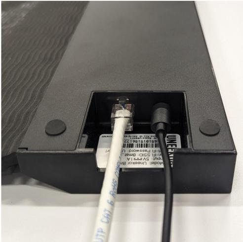
2. Connect Ethernet cable to your PC. Connect USB to your PC or the provided charging block and plug it into an outlet.
