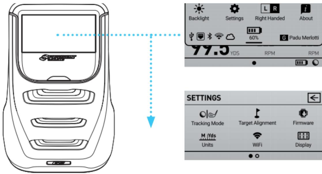
To activate target alignment, swipe down to access the Quick Settings page. Select **SETTINGS**, then go to **TARGET ALIGNMENT**
