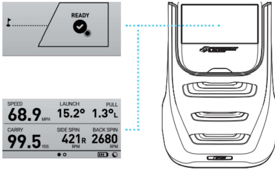
After hitting the ball, the GC3 records your speed, launch angle, push/pull, spin, and carry.
