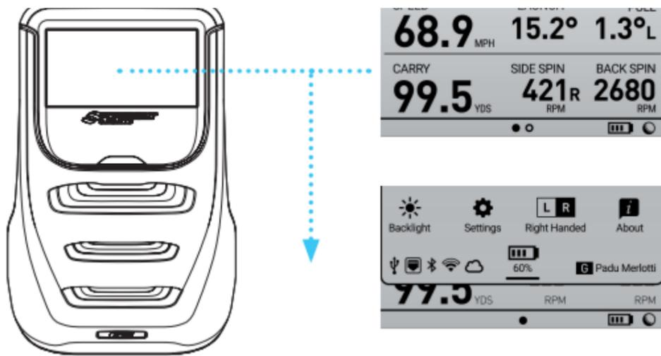
On your GC3 display, swipe down to access the Quick Settings page. On the Quick Settings display, you can access the **BACKLIGHT, SETTINGS, LEFT/RIGHT-HANDED** modes, **ABOUT**, and you can check the battery life
