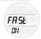
A fast (uncontrolled) ascent is defined as one in which a speed of 12 m/min / 40ft/min or higher was maintained over more than two thirds of the way up. This applies to dives deeper than 12m/40ft only. In such an event, due to the potential of harmful bubble formation, Smart locks the computer for 24 hours in order to discourage you from diving again. In this menu, you have the option to disable the locking up of the computer in the event of an uncontrolled ascent
