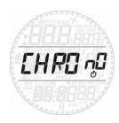
Press and hold the **UP** button to enter this menu. The middle row now features a stopwatch while the time of day has moved to the bottom row. Press the **UP** button to start and stop the time, then press the **DOWN** button to reset the time to zero. Press and hold the **DOWN** button to exit from the stopwatch function (this stops and resets the stopwatch if it was running or stopped at a non-zero value upon exiting).
