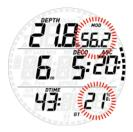
Press the **UP** button while this indication is blinking to initiate the gas switch: the oxygen percentage of G2 starts to blink in lieu of that of G1, and in the top right corner the MOD of G2 is displayed, also blinking.
