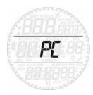
This submenu allows you to download your dive data to a PC or Mac. Press the **ENTER** button and the display will show **PC ready**, symbolizing that Smart is ready to communicate.
