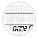
Use the **UP** and **DOWN** buttons to increase/decrease the depth in 3m / 10ft increments
