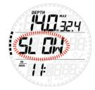
If the ascent rate exceeds 12m/min / 40ft/min at a depth below 12m / 40ft, iblinks as well. If a speed in excess of 12m/min / 40ft/min is maintained for two thirds or more of the depth at which the alarm was first triggered, Smart considers it a dive violation and the display will show the steady if.
