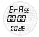
Smart allows you to reset the desaturation in the computer. Any tissue saturation information from a recent dive will be reset to zero and the computer treats the next dive as a non-repetitive dive. This is useful when the computer is loaned to another diver who has not dived in the last 24 hours.
