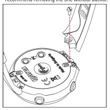
Remove the two screws near the padlock symbols. These hold the battery cover in place.
