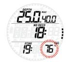
When the oxygen toxicity level approaches 100% the alarm is repeated for 5 seconds in one-minute intervals after the first occurrence and for as long as the value of CNS stays at or above 100%. Consider terminating the dive immediately!
