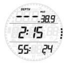
If you submerge again before the 3-minute countdown is over, the dive time will resume from where it left off, including the time spent on the surface. If you do not submerge before the end of the countdown, Smart considers the dive finished, records the data to the logbook and reverts to the so-called post-dive mode.
