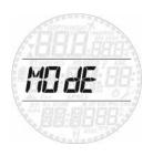
Here you can define the type of gas you will be breathing during the dive (air or enriched air nitrox, including multigas). You can also set Smart to bottom timer (BT), in which case Smart will show only time, depth and temperature: it will not carry out any decompression calculation and it will not show any warnings and alarms. You can set Smart also to APNEA, which in essence is a bottom timer with special features dedicated to apneists.
