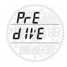
Press and hold the **UP** button to enter this menu and put Smart into the ready-to-dive mode.
