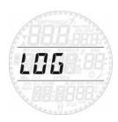
Smart can record the profiles of approximately 35 hours of diving, at a sampling rate of 5 seconds. The information can be transferred using the optional USB clip to PC via the Dive Organizer software or to a Mac via the Divers' Diary software. In addition, Smart can show most of the information directly on the display.
