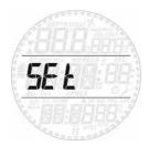
Smart's **SEt** menu allows you to change settings. Once inside this menu, press the **UP** or **DOWN** button to scroll between two submenus: **SEt dIVE**, where you can set parameters pertaining to the dive, and **SEt tIME**, where you can set parameters pertaining to time and date.
