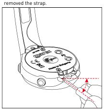
d) Remove the cover then remove the o-ring.
