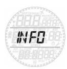
This submenu provides information about the hardware and software of your Smart and about the status of the battery: **OK** means the battery is good, **LO** means the battery is weak but you can still do a few more dives, and **KO**
