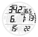
By pressing the **UP** button, you can modify the information displayed in the upper row. At each button press, the screen cycles through, max depth, average depth, MOD (nitrox only), deep stop (if activated and if calculated to be present), and an empty field.
