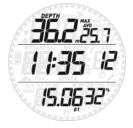
Press and hold the **UP** button to view the next page of the dive log, which shows the surface interval prior to the dive alternating with the dive time and **CNS** (alternating between start and end value) in the bottom row. In case more than one gas was used in the dive, information about **G2** and **G3** if applicable is shown alternating with G1 on the first page.
