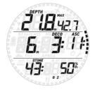
If you press the **UP** button while G2 is blinking, the next available gas in the list will be displayed instead. This will be G1 if only two gases are set or if you are deeper than the MOD of G3, or G3 if you have set three gases and are shallower than the MOD of G3.
