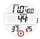
In this case, if the diver attempts a repetitive dive after surfacing, Smart will only function as a depth gauge and timer (bottom timer mode), and will display on the screen throughout the dive.
