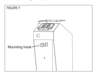
**3** Remove the bracket by sliding it down and off the safe (see Figure F).
