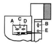
Install hinges on door using screw slot (A) or (D). Install all doors on cabinet using only screw (B) - then adjust all doors for fit. Then install the remaining screw in (E) on the stile and in (C) or the remaining adjustment slot on the door. (Recommended minimum face frame size is 1-1/2 inches)
