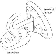
1. Assemble the catch as shown to the above right. Slide the latch into the mounting base from the back. The hook must point down. You may wish use tape to temporarily hold the latch into the base so as to
