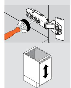
NOTE: On non-cam mounting plates, loosen screws, adjust door and retighten screws
