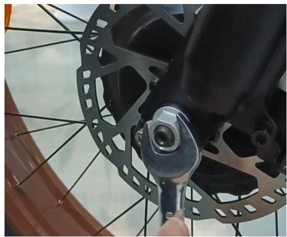
10. Put the nut into the motor axle and tighten it by wrench, first tighten the nut on the disc brake side, and then the motor cable side
