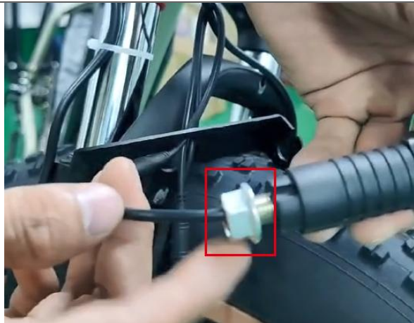
23.Loosen the nut of one turning lights
