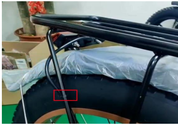
37. Use cable ties to fix the rear light cable on the rack
