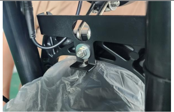
22. Put on the light bracket and tighten the nut by wrench
