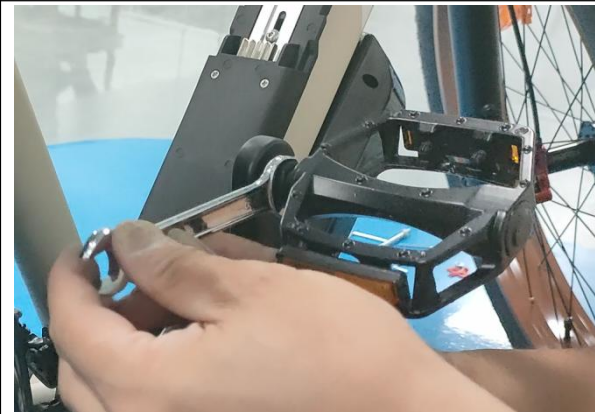
31. Twist in the pedals and tighten the pedals by wrench. Please note the direction of rotation
