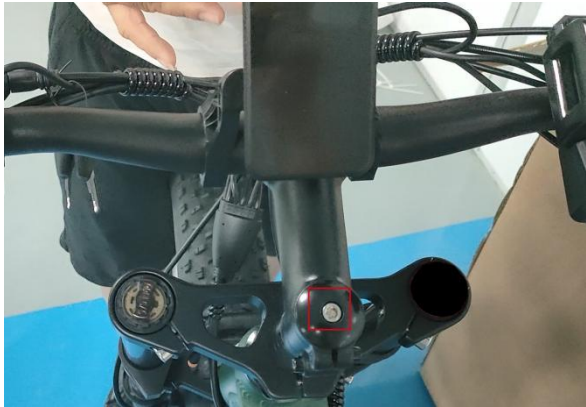
15. Clamp the tire with knees and adjust the direction of handlebars, tighten the top bolt first
