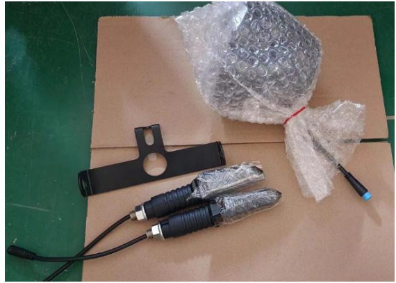
20.Take out the headlight, two turning lights and the light bracket
