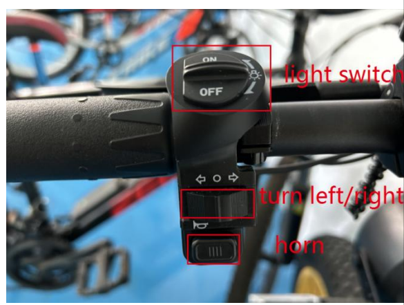
42. Light instructions: ON/OFF button; turn left/right; horn button
