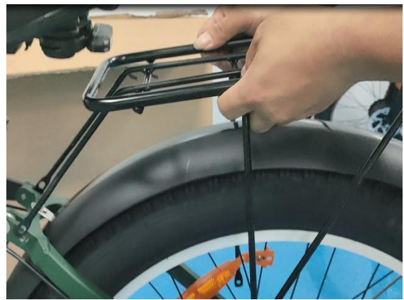
34. Install the rear rack. Some adjustment may be needed for the best fit. The rack prongs can be bent at different angles by force
