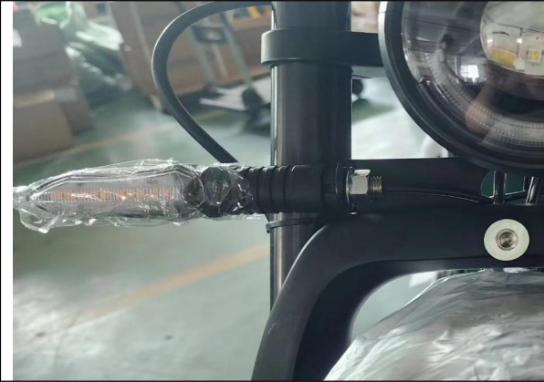
25. Install the right turning light on bracket, put the cable of right turning light through the middle hole of bracket
