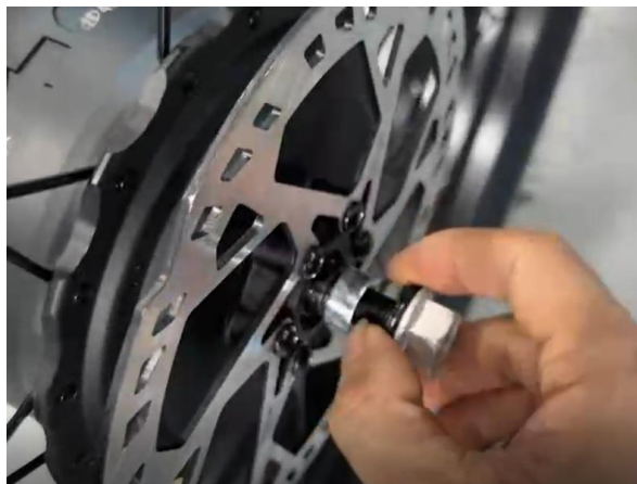
05.Loose the nut on both sides of front motor axle, move the black retaining washer to the end
