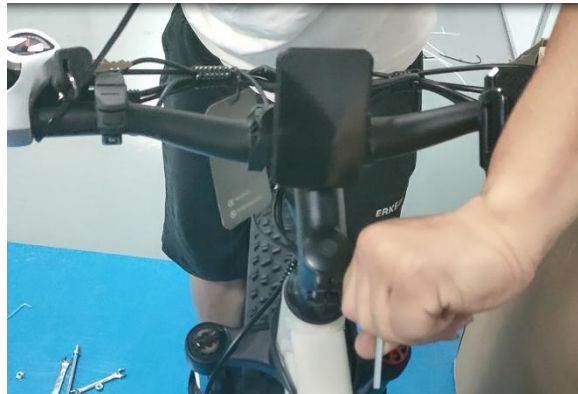
16. Clamp the front tire with knees and adjust the direction of handlebars, tighten the 2 bolts on both sides
