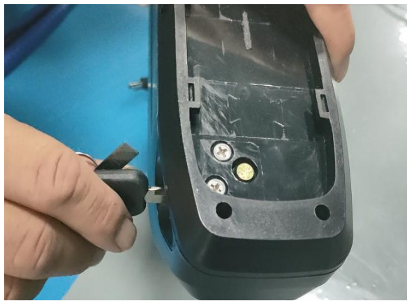
39. Insert the battery key into the key hole
