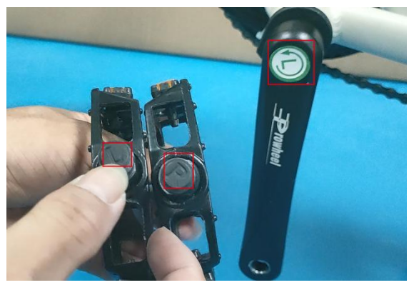
30. Put the Left & Right pedals correctly into the cranks
