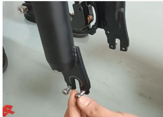
04.Remove the 4 screws on the bottom of the fork
