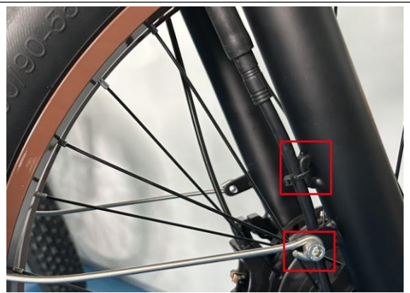
30. Fix the front motor cable to the fork with a cable tie. Fix the front fender support to the fork
