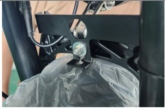
22.Put on the light bracket and tighten the nut by wrench
