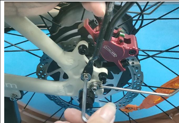
33. Tighten the lower bolts first
