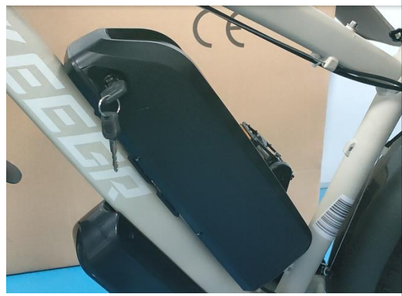
40. Put the battery on the frame and lock it. Ensure the battery is locked tightly on the frame
