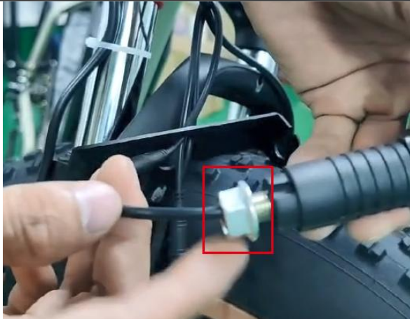
23. Loosen the nut of one turning lights
