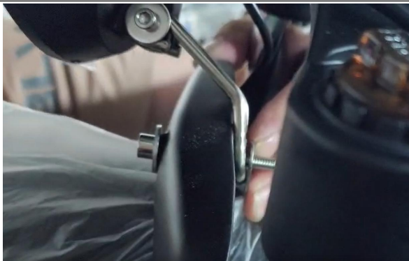
21. Put the headlight and then front fender on the fork
