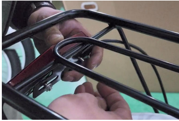
37. Install the rear light on rear rack, tighten the nuts by wrench
