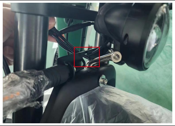
26. Put headlight cable through the middle hole of bracket.
