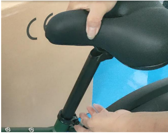
31. Insert the seat post, tighten the nut and quick-released lever
