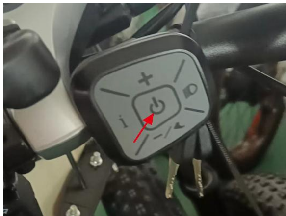
41. Press the ON/OFF button for 2-3 seconds to turn on the LCD display, now you are ready to go
