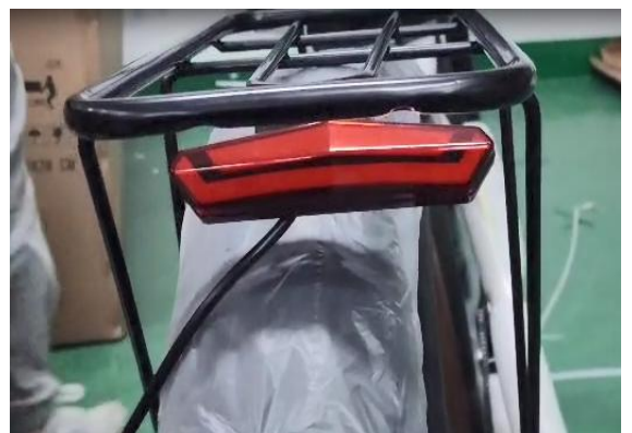
36. The rear light should be installed like this
