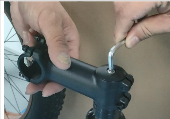
03.Tighten the top bolt
