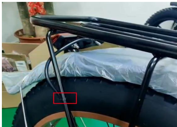
37. Install the rear light on rear rack, tighten the nuts by wrench
