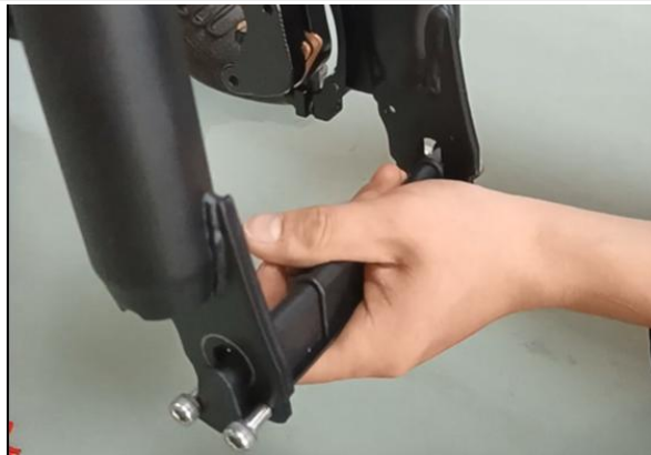
03.Remove the retainer that protects the fork from deformation
