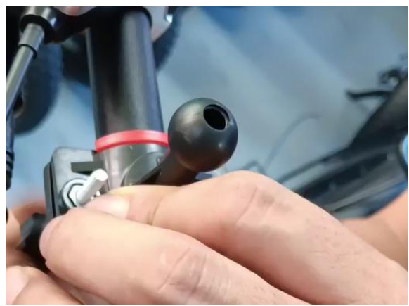
18. Install the bracket on the handlebar, tighten the screw
