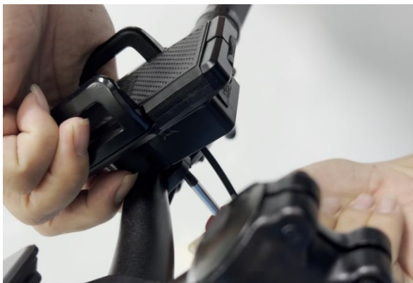
17. Install the phone holder on the right side of handlebars (there is a USB charging port on the bottom to charge the mobile)
