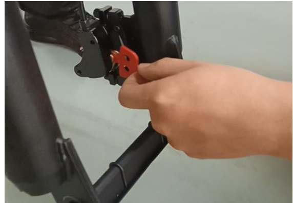
02.Remove the red spacer in the caliper on the front fork
