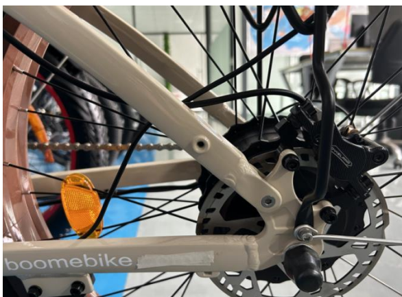
35. Tighten the lower bolts first
