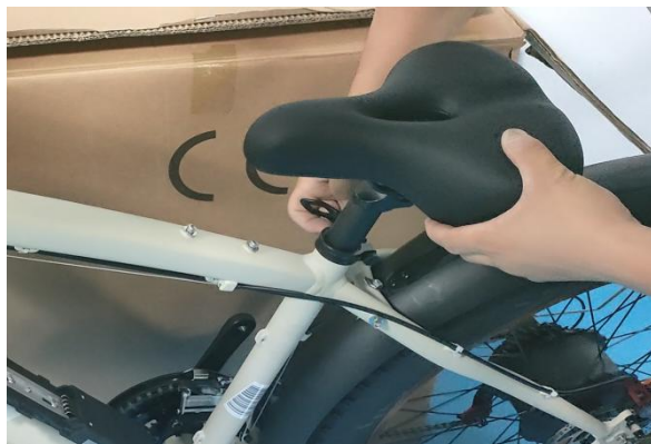
29. Insert the seat post, tighten the nut and quick-released lever
