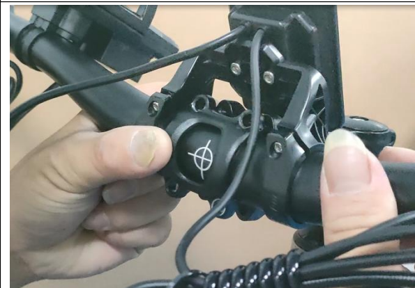
05.Fit the stem and handlebar together
