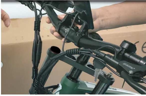
13. Fit the stem and handlebar together
