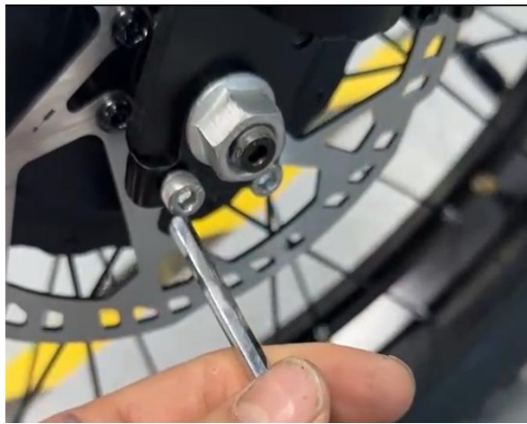
09. Twist in and tighten the 2 small screws by tool at the bottom of fork on both sides
