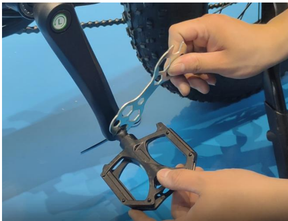
33. Twist in the pedals and tighten the pedals by wrench. Please note the direction of rotation
