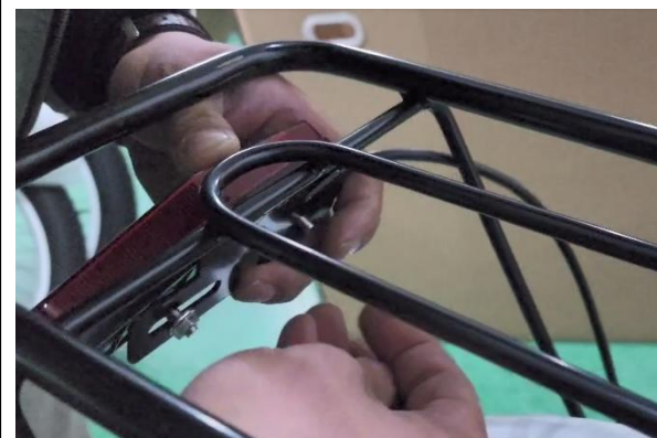
35. Install the rear light on rear rack, tighten the nuts by wrench
