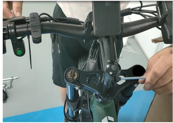
16. Tighten the 2 bolts on left and right sides
