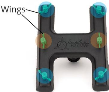
Rotate the spray jets on the T24 manifold so that the two center "wings" highlighted orange are straight. The corner jet "wings" highlighted blue should be turned to 45 degree angles. Use the picture for reference.
