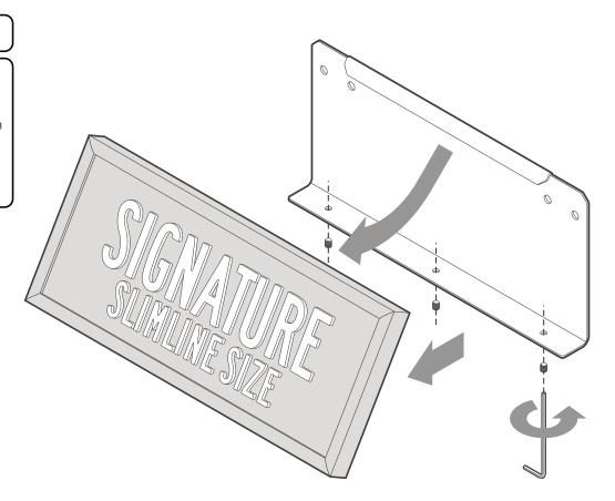
ASSEMBLE TOP AND BOTTOM MOUNTS TO BRACKET
