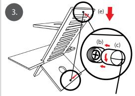
Screw 1st silver cap (c) by hand, onto the top brass bushing (b). Next, Pull and bend the top of the ladder panel (e) downwards in order to screw and tighten the bottom silver cap (c) onto the brass bushing (b).
