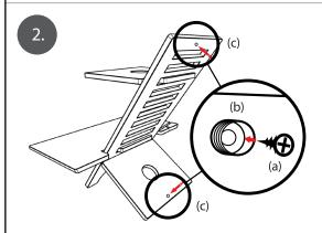
Using a star screwdriver, insert the 2 x screws (a) into the 2 x brass bushings (b) and then screw them into your center point dots (c) as shown above.
