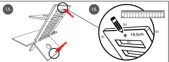
Turn your DeskStand around so that the rear is facing you. Measure and mark the center points at the top of ladder panel and bottom of the base panel as shown above. Measure 19.5cm from the side edges (a) and 2,5cm from the top and bottom edges (b) and draw a dot.
