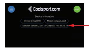
To control your chiller remotely, you will need to copy this IP Address onto any web browser on your smartphone, tablet or computer.
