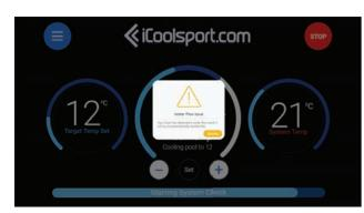
It can occur if air is trapped in the water pipes or in the pump, or if flow is restricted in the hoses by some sort of blockage. There could be an air leak in the hoses or pipes from the pool or trapped air in the system.
