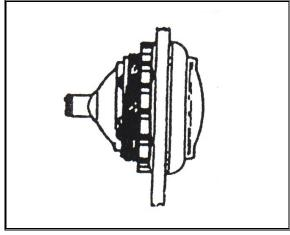
Your USA Spa has a standard 12v light. The spa light may be turned ON or OFF by pressing the LIGHT button, located on the spa side control. The light will automatically turn off after 4 hours.
