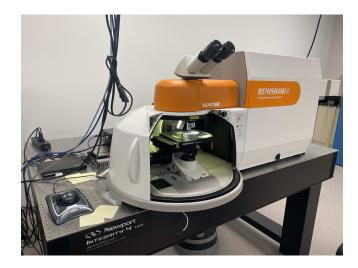
FIG. 1. Digital photograph of the Renishaw inVia<sup>TM</sup> confocal Raman microscope used in our experiments.
