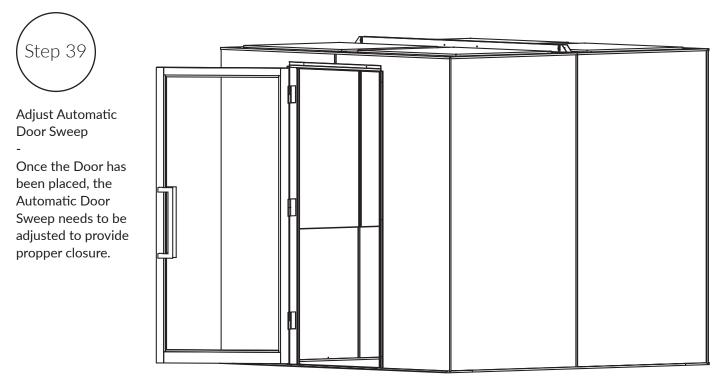
Start by dialing the plunger in clockwise direction to allow for more Door Sweep drop.
